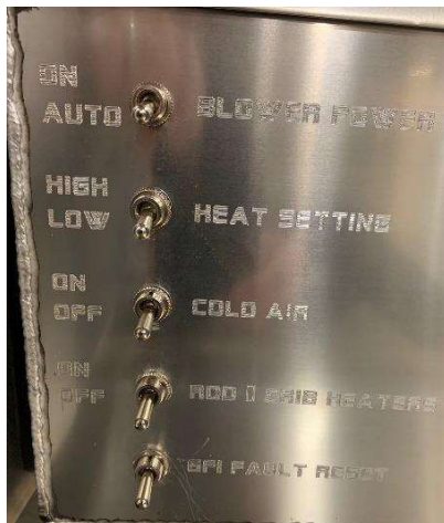
Fig. 6 Control Switches Model RRSHA5 Shown with Optional Rod/Crib Circuit & GFI
