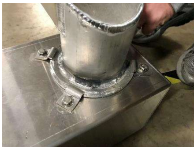
Fig. 325 Nozzle Installed with Clips Turned In
